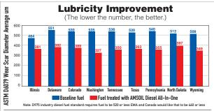
The ASTM D975 diesel fuel standard specifies a wear scar below 520 µm in ASTM D6079 testing, while the Engine Manufacturers Association (EMA) specifies a wear scar below 460 µm. Testing reveals AMSOIL Diesel All-In-One provides significant lubricity improvement in diesel fuels found across the U.S., delivering improved wear protection.
